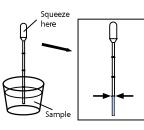
Draw nasal wash or nasal aspirate sample to the **first** (lowest) mark of the graduated transfer pipette.
